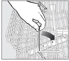
The positioning rail can be flipped over to the middle of the basket for easy sorting and removing of crockery.
